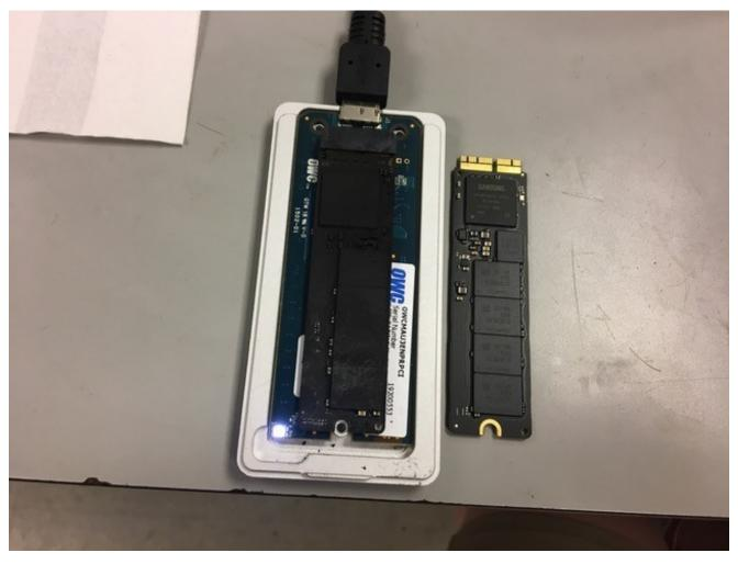
Even though the SSD was right next to the ruptured cell and got very hot, we were able to recover most of the data from it!
